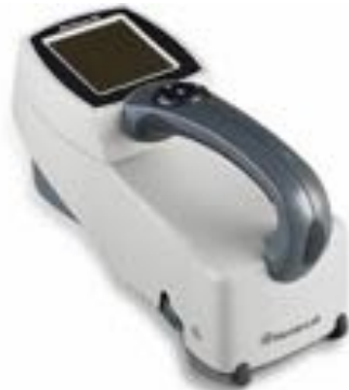
Portable colorimeter (MiniScan EZ 4500L, HunterLab, USA)
