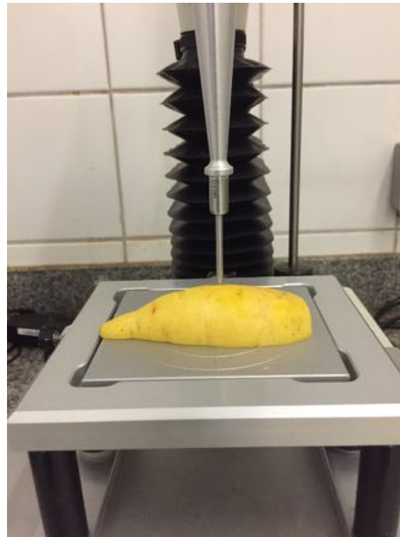
TA.XT Plus Texture Analyzer (Stable Micro System, Surrey, UK)
